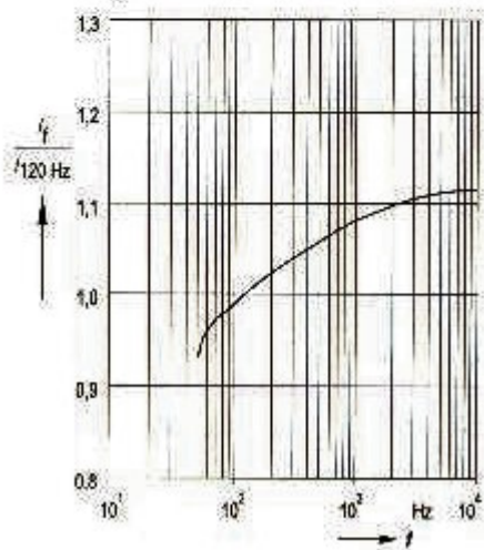
Permissible ripple current i_{ac} versus frequency f V_R \geq 160 Vdc
